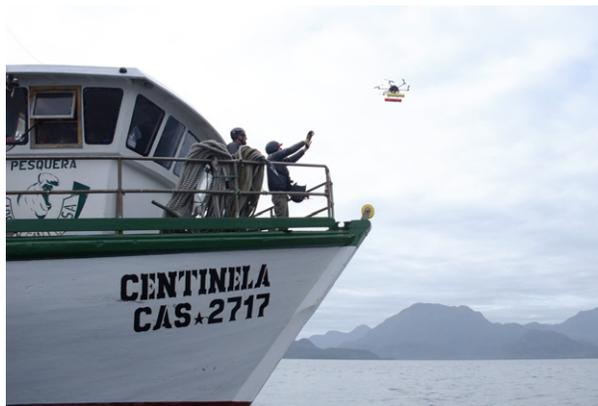
Figure 2. Photograph of the hexacopter being hand retrieved from the foredeck of the 18.6 m wooden boat by a ground station operator (MM) with pilot (JD) close by.
